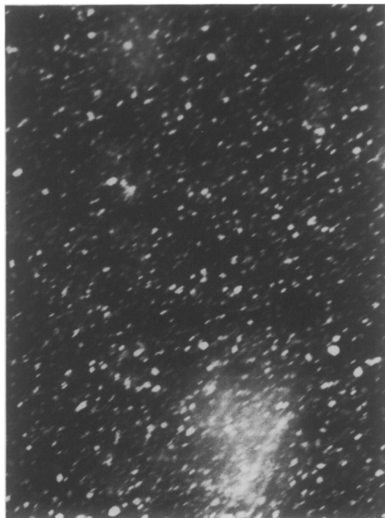
Figure 7 STEM dark-field image of n-beam reflections of a quench-cooled iPP sample. Magnification 50\,000\times ( 1\text{ cm}=0.05\ \mu\text{m} )
